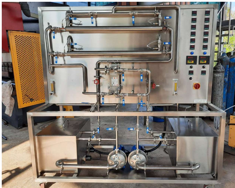
Figure 1 Heat Exchanger Apparatus
