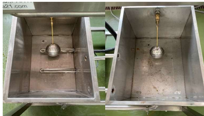
Figure 3 hot water tank (Left) and cold water tank (right).
