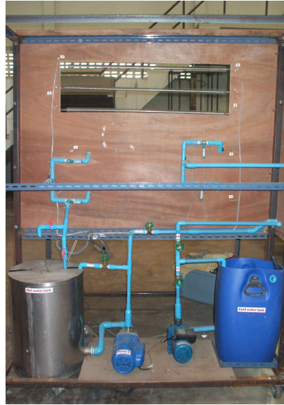
Figure 4 Back view of Heat Exchanger
