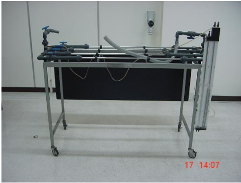
Flow in Pipe Network
