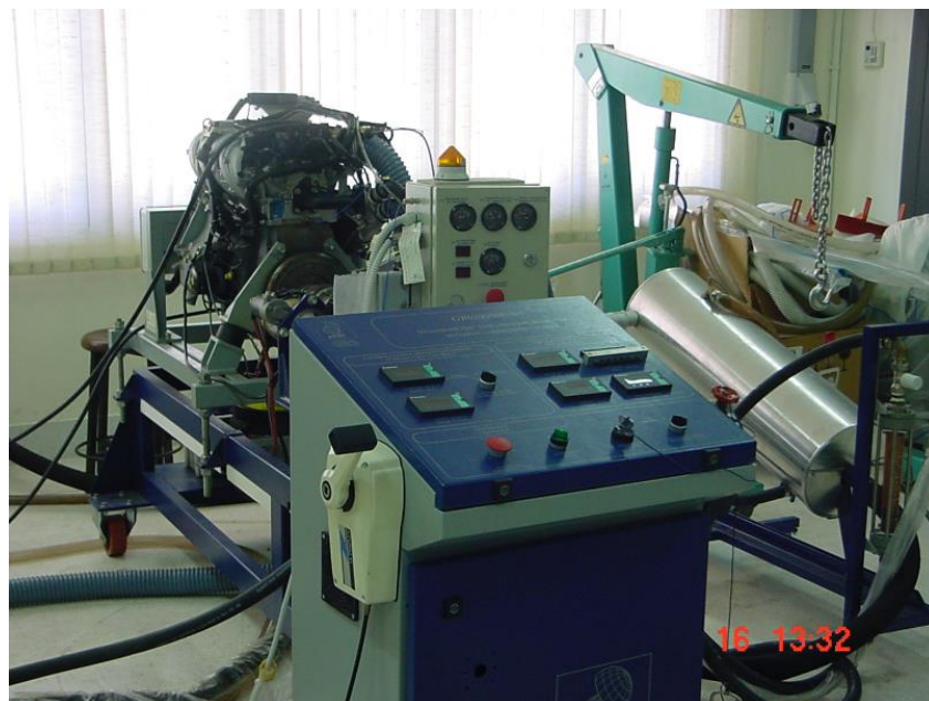
Gasoline & Diesel Engine Test
