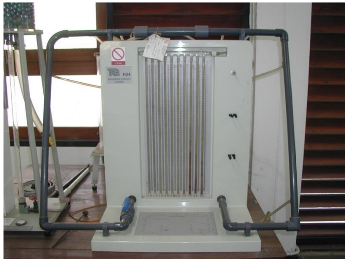
4.5 Pipework Energy Losses
