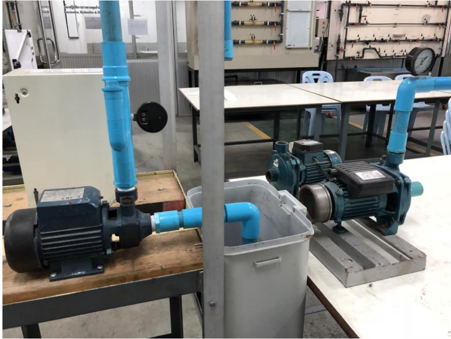
Centrifugal pump Test Set
