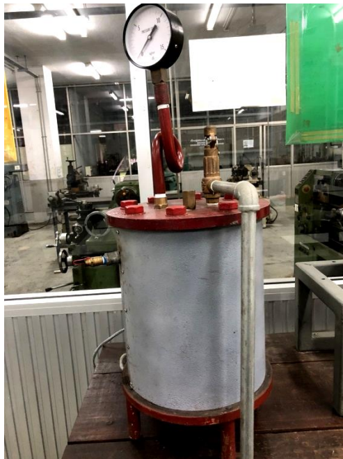
Boiler Test set
