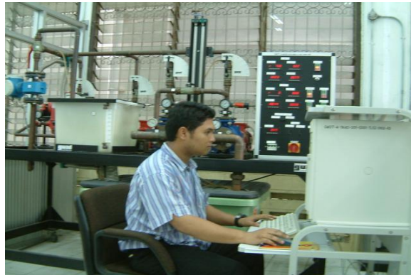
1.1 Pump Testing Rig
