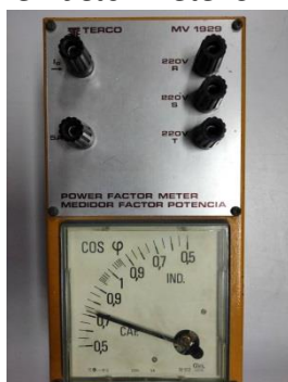
23. Power factor meter 5 A MV 1929
