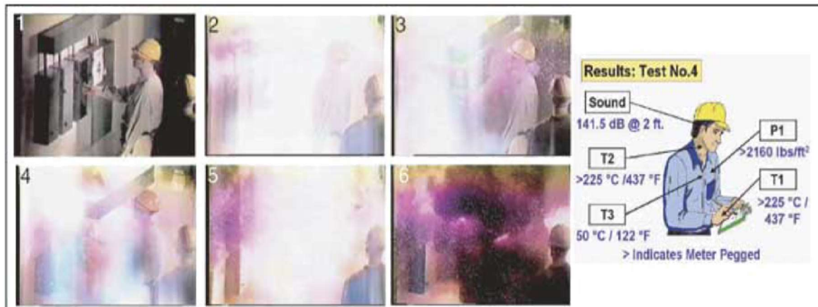
Figure 3. Test 4 - 22,600 - A rms, 480-V, fault initiated on line lug of size 1 starter, feeder protected by a 640-A noncurrent-limiting overcurrent protective device, and fault was cleared in 6 cycles.
