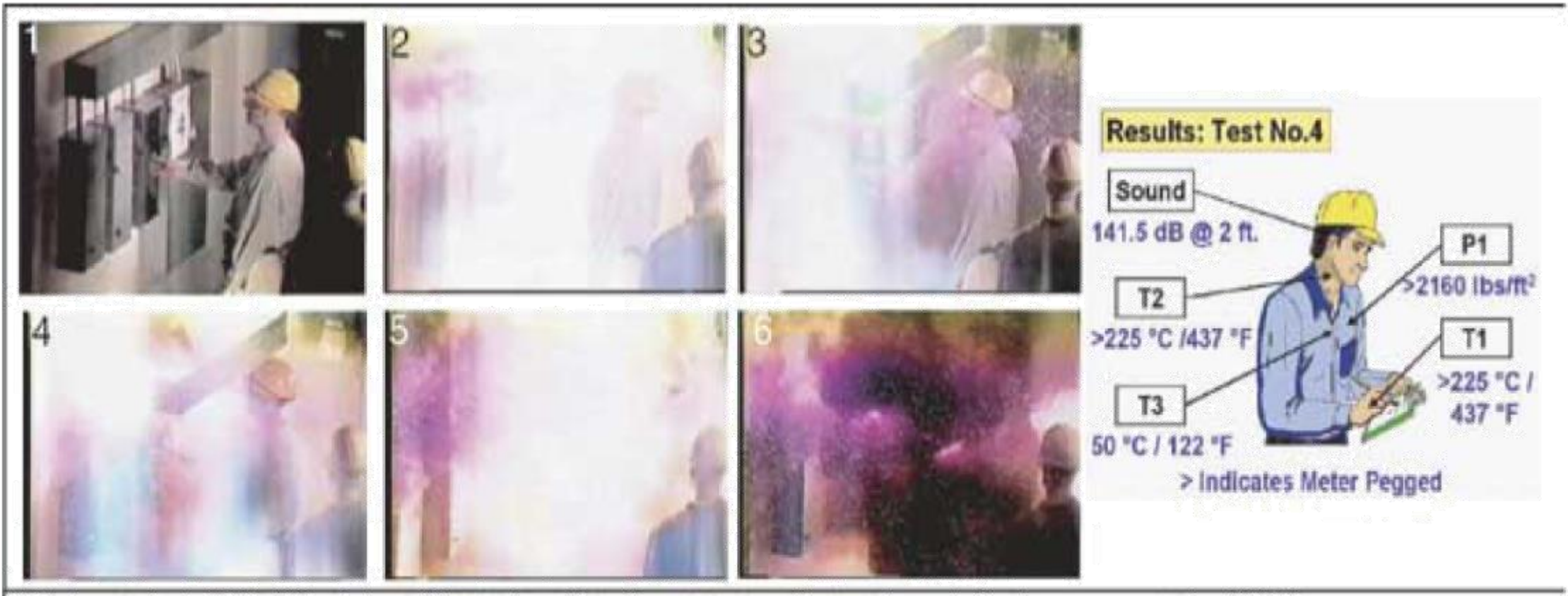
Figure 3. Test 4 - 22,600 - A rms, 480-V, fault initiated on line lug of size 1 starter, feeder protected by a 640-A noncurrent-limiting overcurrent protective device, and fault was cleared in 6 cycles.
