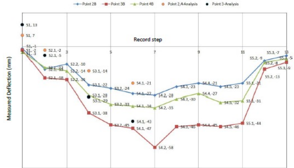
Figure 3.8 Plots of measured deflection and analysis results for each construction stages for Main gantry B
