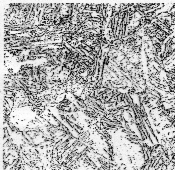
Fig. 80 15-5PH martensitic precipitation-hardenable stainless steel (41 HRC), solution annealed and aged. Structure is tempered martensite. Vilella's reagent. 200×
