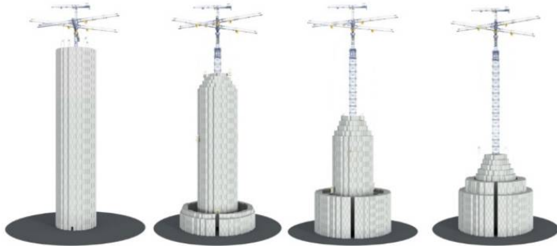
The left-most image shows the system in its fully charged state; the images to the right show various stages of discharge. (Source: Energy Vault)
