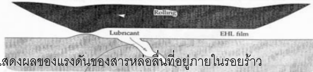
2) Lubricant forced into crack by extreme pressure
