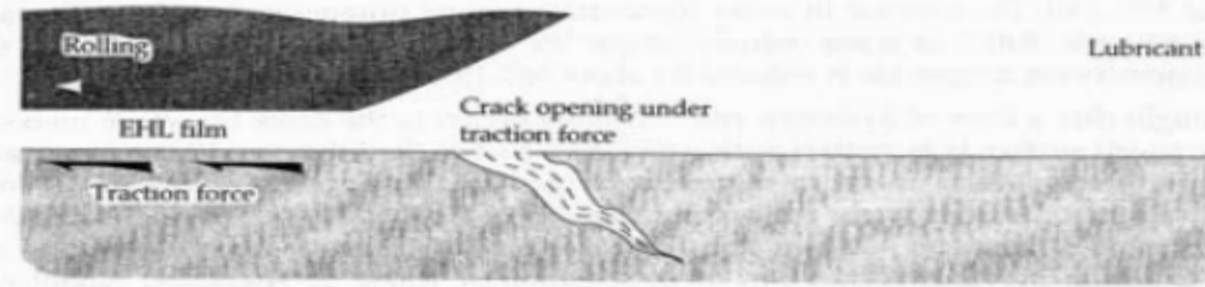
1) Crack opening under lateral tensile stress
