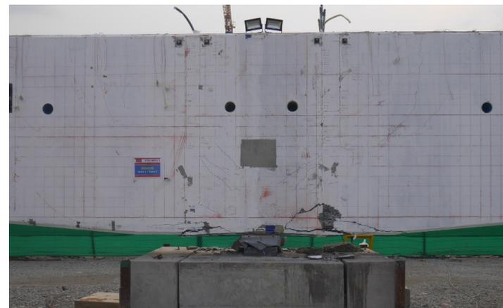
*Cracking pattern at the pier segment.*
