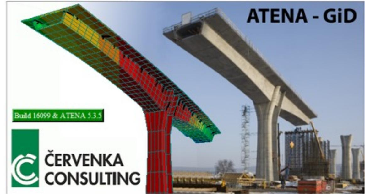
With ATENA You can simulate real behavior of concrete and reinforced concrete structures including concrete cracking, crushing and reinforcement yielding. ATENA gives you the power to check and verify your structural design in a user-friendly graphical environment. ATENA program is proved by over 1000 installations worldwide. A typical ATENA finite element model of bridge structure is shown in figure
