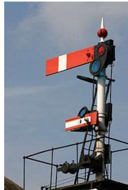
A British semaphore stop signal with subsidiary arm below.
