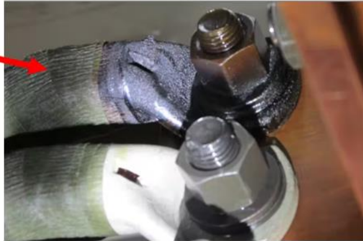
Figure 1. Hydrogen was generated in the transformer oil because of overheating on a low-voltage bushing connection owing to a loose nut on a 500-MVA generator step-up transformer. A hydrogen monitor alerted the owner to the problem. The transformer was repaired on-site.
