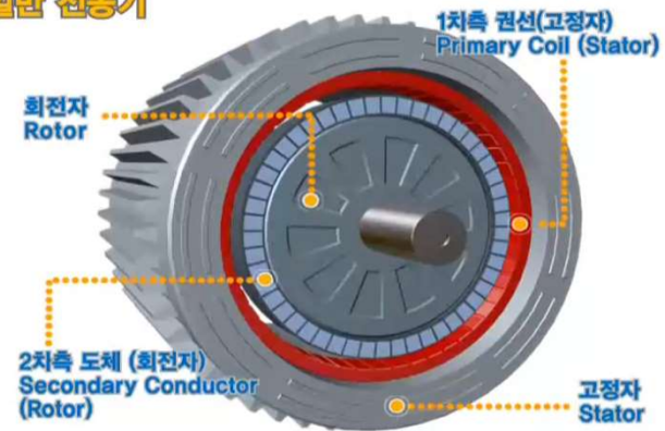
LIM (Linear Induction Motor)
