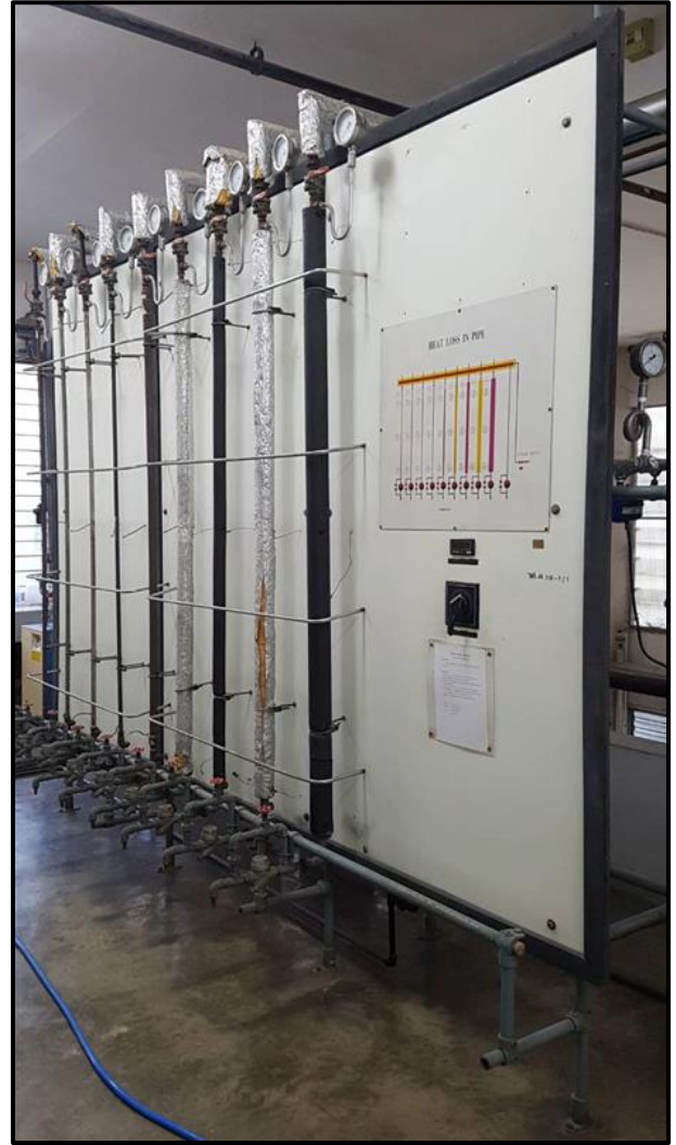
2. Heat Loss from Pipe
