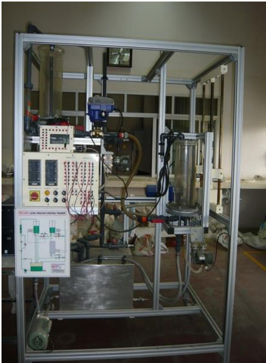
Level process control trainer
