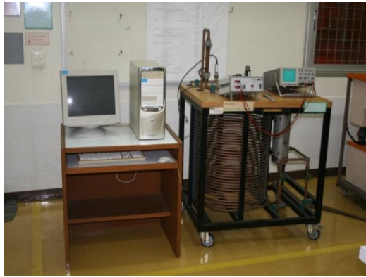
15. Water Hammer Apparatus
