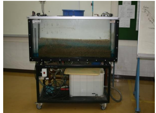
16. Drainage and Seepage Tank
