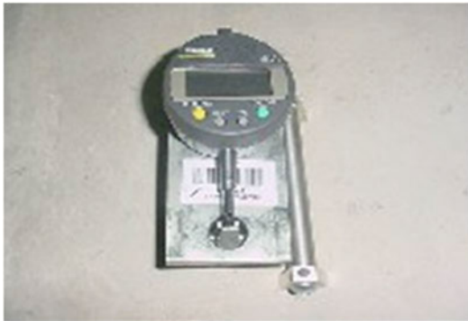
25. Digital Crack Measuring Gauge
