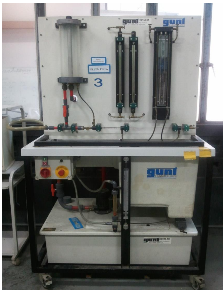
Flow and Fiction Loss in Pipe
