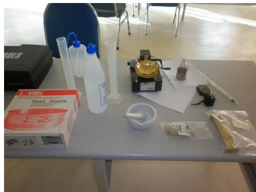
(2) ชุดทดสอบ Atterberg's Limit
