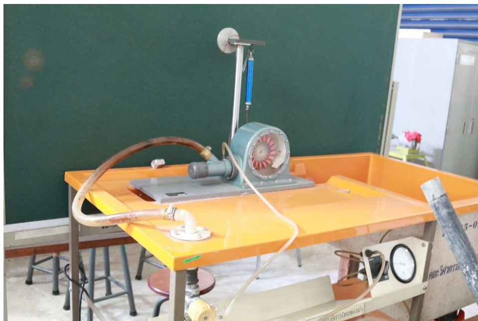
Pelton Wheel Turbine Test Set
