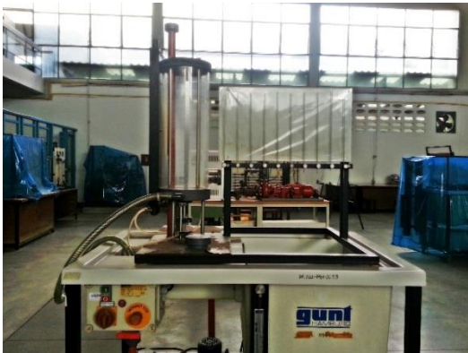
Exp No.3 Flow through of Orifices and Weirs
