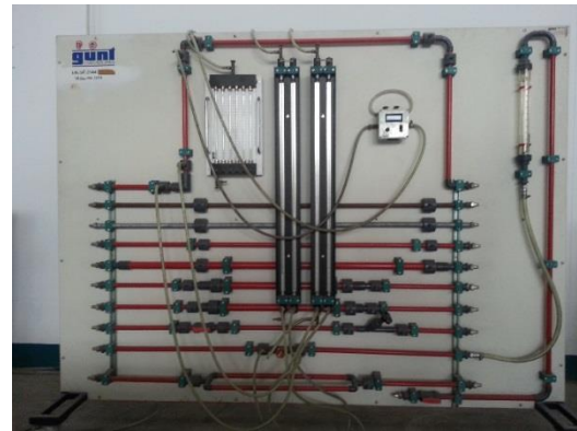
Exp No.4 Flow in Pipe
