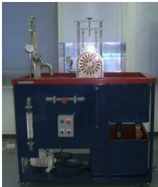
Multi Turbine Test Set
