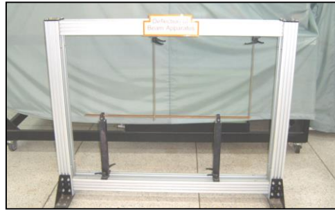
2. Deflection of Beam Test Set
