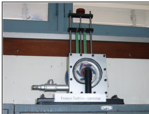
2. Pelton &amp; Francis Turbine Set
