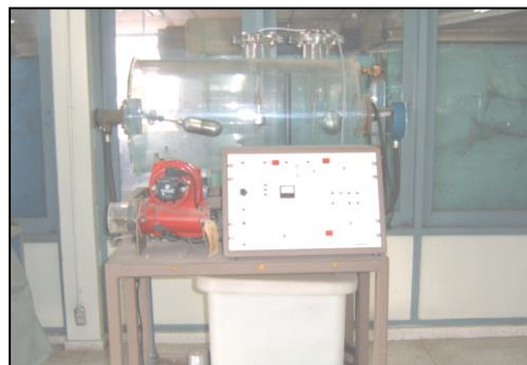
4. Boiler Demonstration Unit
