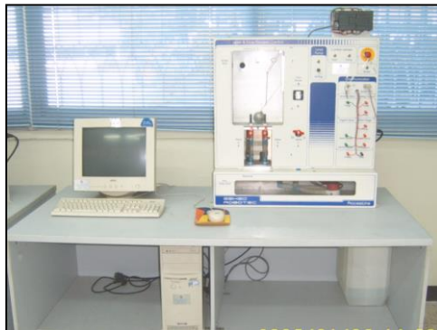
8. Level & Flow Process Control Test
