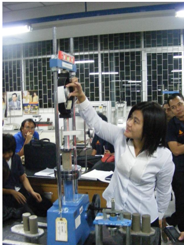
ชุดทดสอบ Unconfined Compression Test
