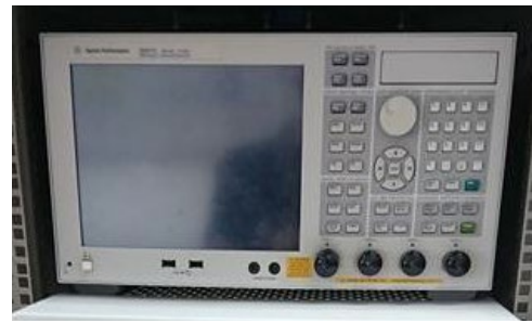
Network Analyzer 300kHz-14GHz (Tx, Rx Mode) z (Tx and Rx Mode)
