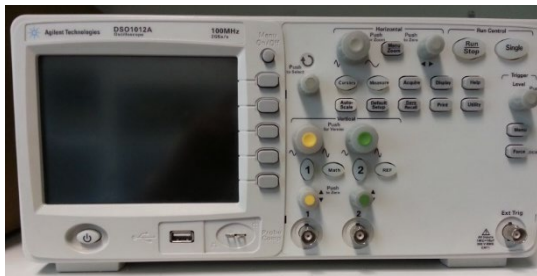
Digital Oscilloscope DSO1012A 100MHz
