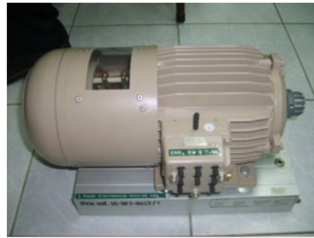
Three-Phase Synchronous Machine
