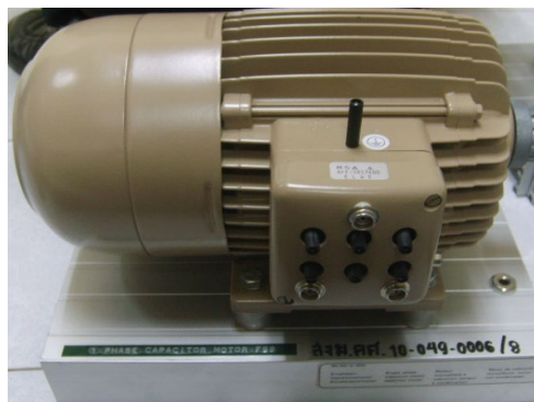
Single-Phase Induction Motor with Auxiliary Starting Winding
