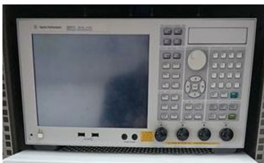
Network Analyzer 300 kHz–14 GHz (Trans. Mode)
