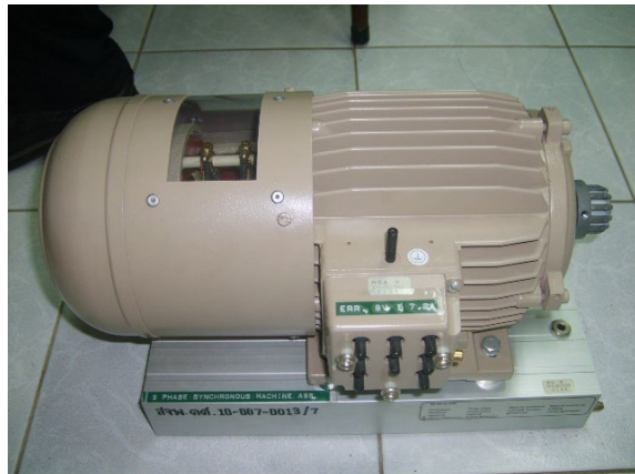
Three-phase Synchronous machine
