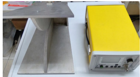
Horn Antenna+Signal generator (9 kHz – 6.1 GHz)
