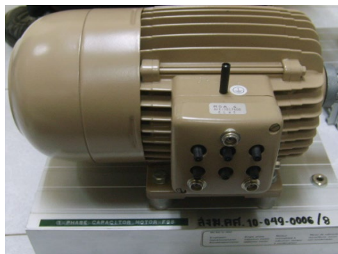
Single-Phase Induction Motor with Auxiliary Starting Winding
