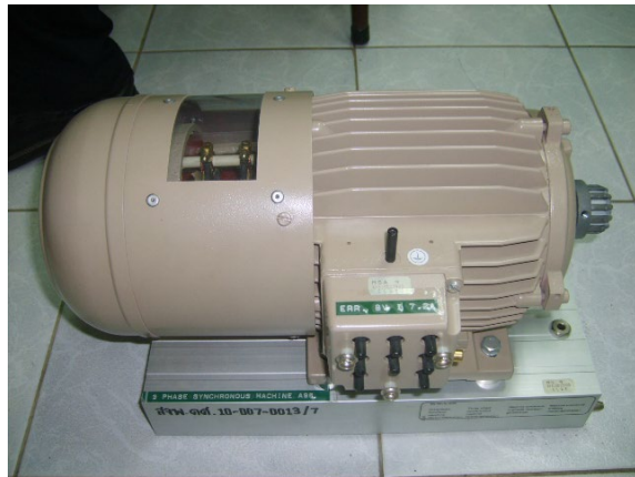
Three-phase Synchronous machine
