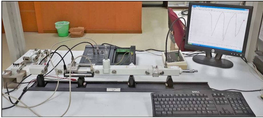
Figure 5.42: Lucas-Nulle (LN) Equipment for analyzing Microwave Behavior; measurements at short, open and matched load.
