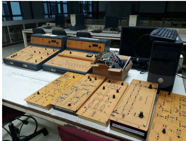
Figure 5.33: Experimental sets of De Lorenzo Modules: Transmission Line Trainer, PCM Trainer, Modulation Trainer, Digital Transmission Trainer etc.
