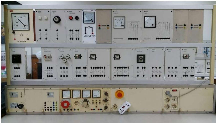
Figure 5.11: 1-phase, 3-phases power supply with adjustable AC and DC settings (Set #2)
