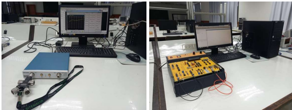
Figure 5.43: Network Analyzer and Optical Fiber.
