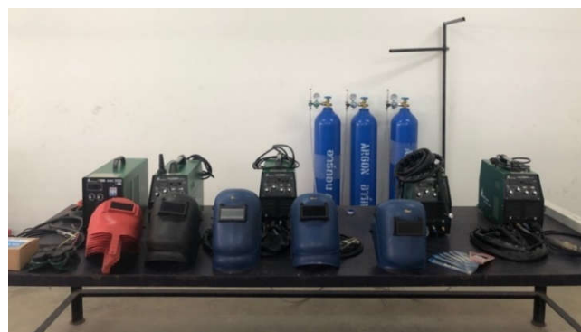
Welding machine & Welding equipments (Argon tank, face shields, goggles, etc.)
