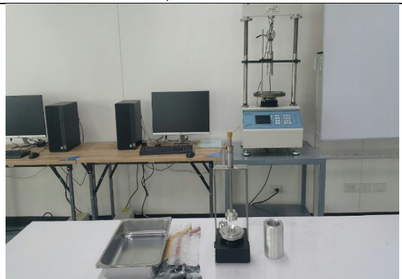
12. Unconfined compression test
