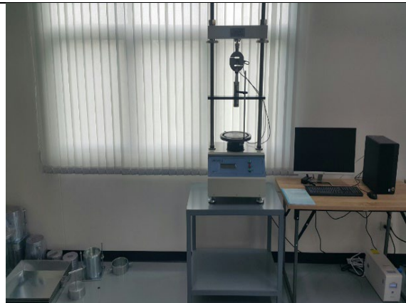
12. Unconfined compression test
