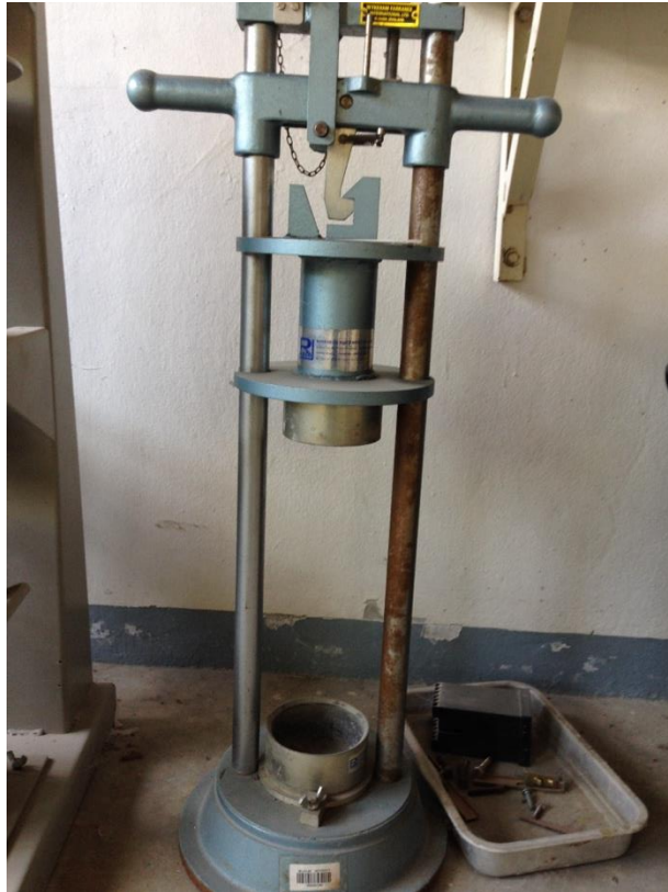
Penetration Value Testing Machine
