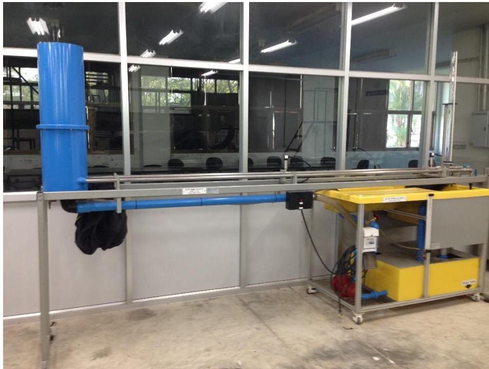
ชุดทดสอบ Water Hammer and Surge Tank
