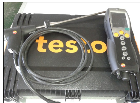
Combustion efficiency measurement set
