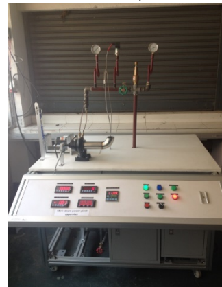
Mini-steam power plant apparatus
