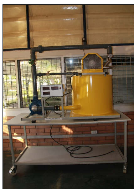
Pelton turbine apparatus
