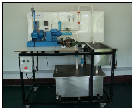
Centrifugal pump apparatus
