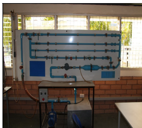
Loss of Energy in pipe apparatus
