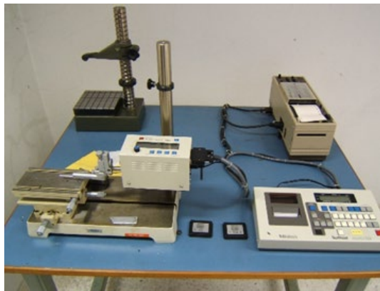
Surface Roughness Test station/Portable Surface Roughness Tester
