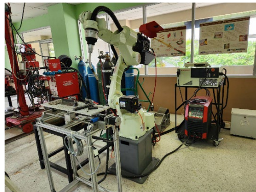
Robotic Welding Machine
