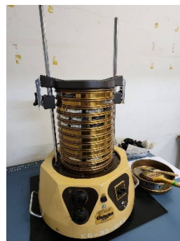
Sand Distribution Testing (A.F.S. No. testing)
