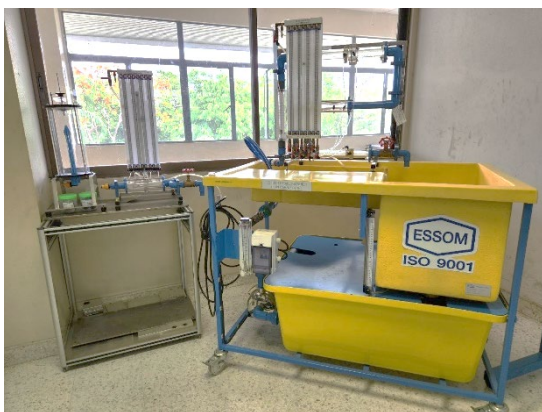
Hydraulics Bench with Bernoulli's Theorem Apparatus, Flow Meter and Impact of Jet
