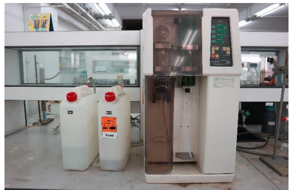
Distillation Unit (Ammonia),
