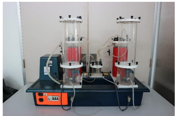
Aerobic treatment unit
