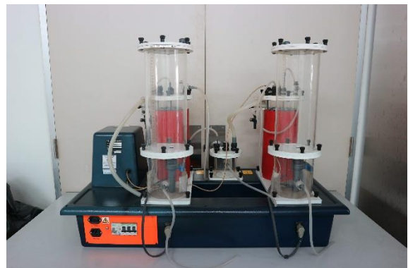
Anaerobic treatment unit
