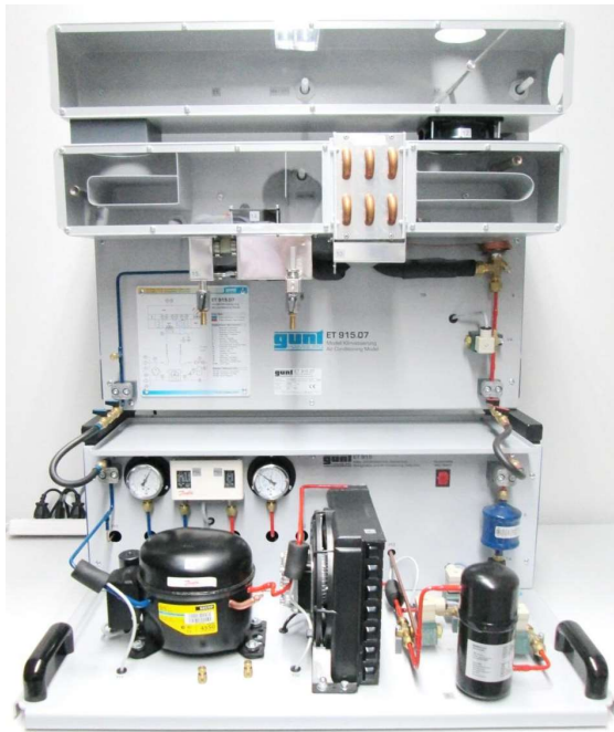
(4) Refrigeration and Air Conditioning Unit
