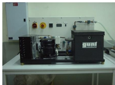
Heat Exchanger Apparatus
