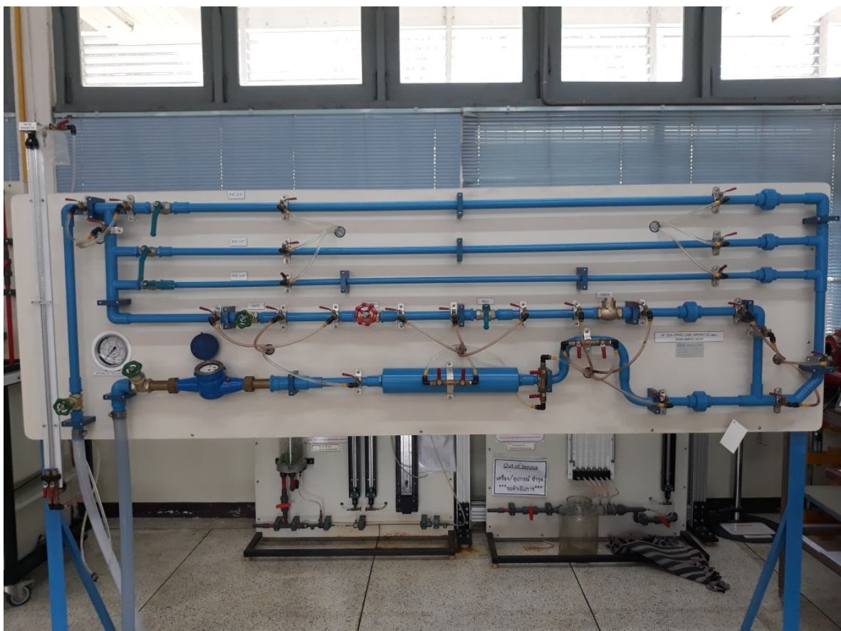
1.6) Flow or Friction Loss in Pipe
