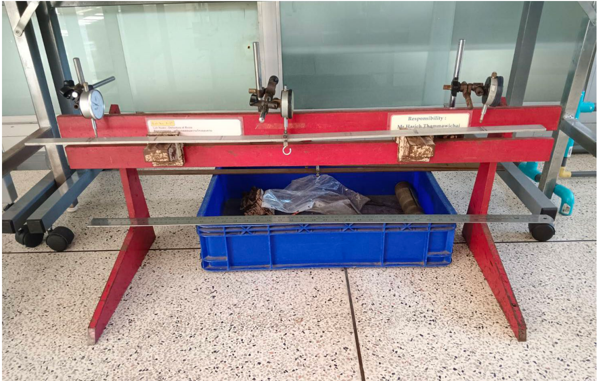
5.2) Deflection of Beam Test Set
