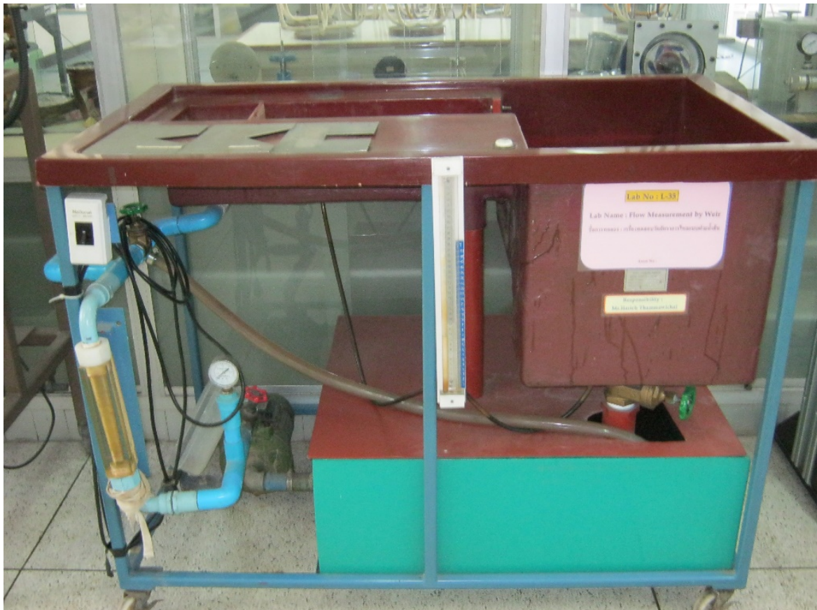
1.9) Flow measurement by weir
