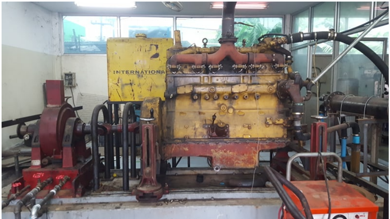
2.2) Engine Horsepower Test
