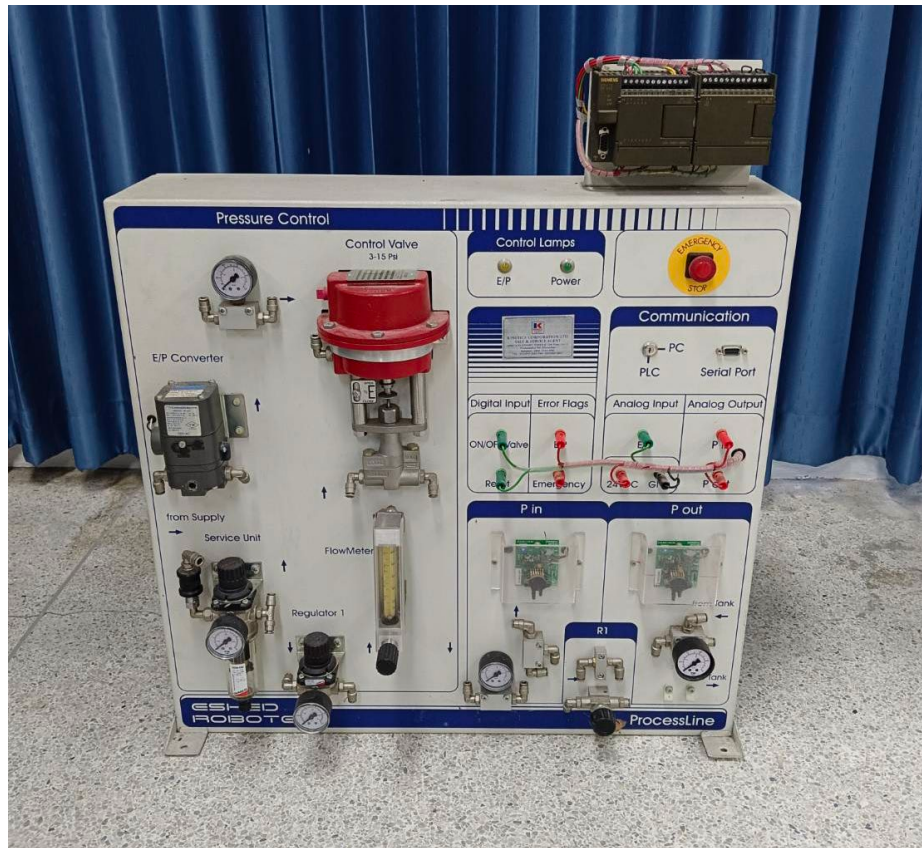
4.6) Pressure Control Test
