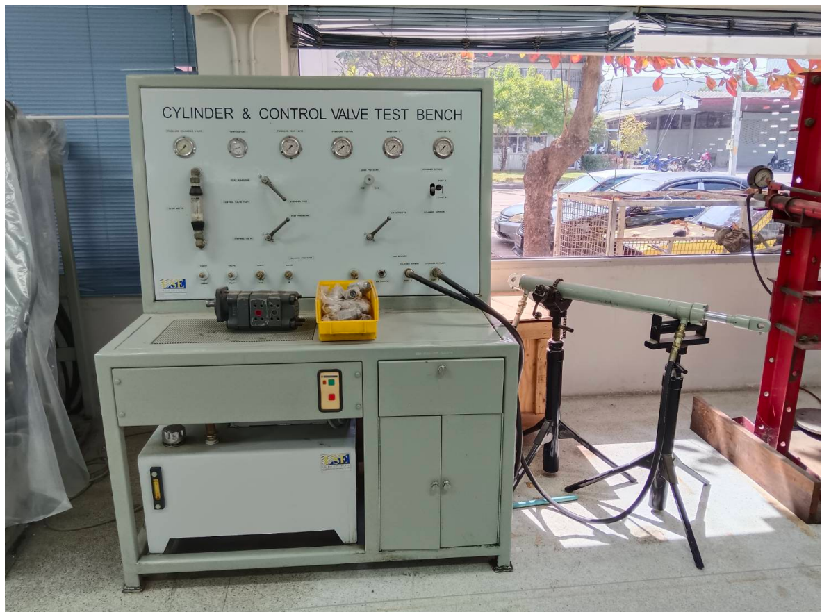
1.8) Hydraulics Cylinder & Valve Test
