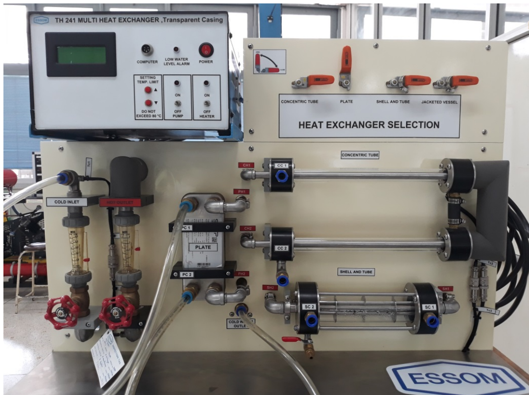
3.12) Heat Exchanger selection
