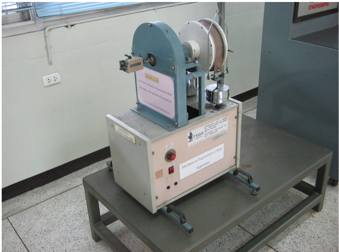
3.6) Mechanical Equivalence of Heat
