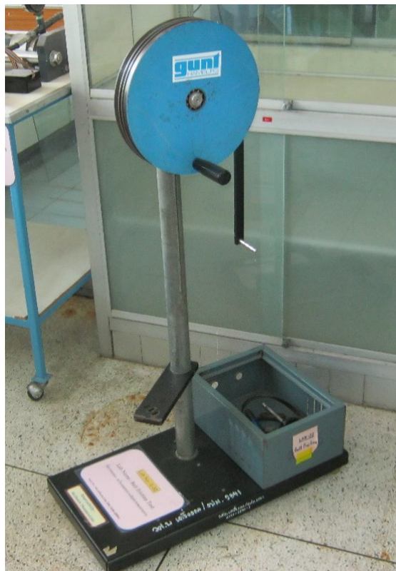
5.1) Belt Friction Test
