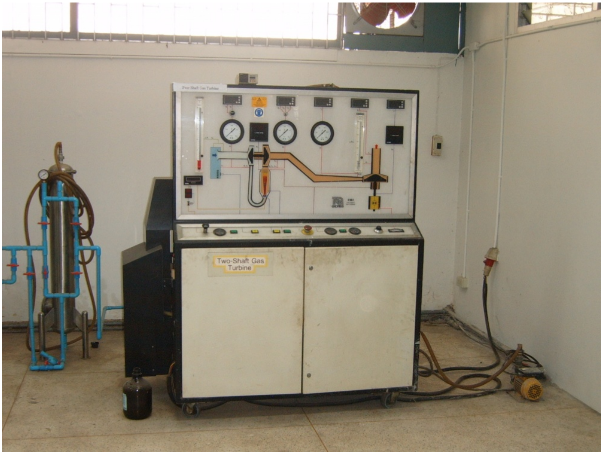
3.5) Two Shaft Gas Turbine
