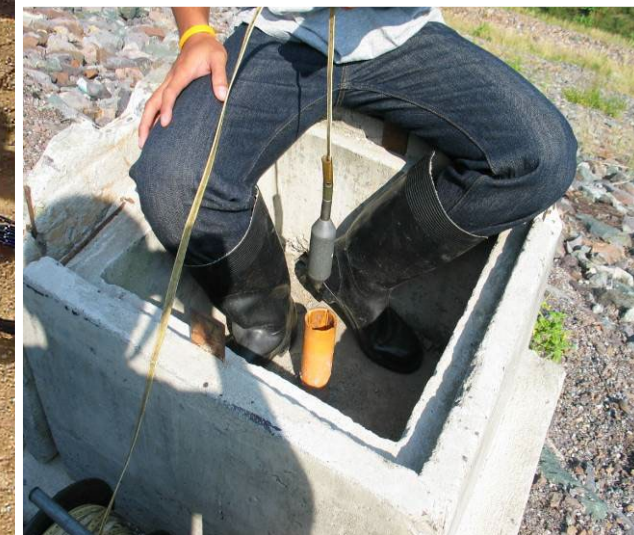
Magnetic Settlement Probe
