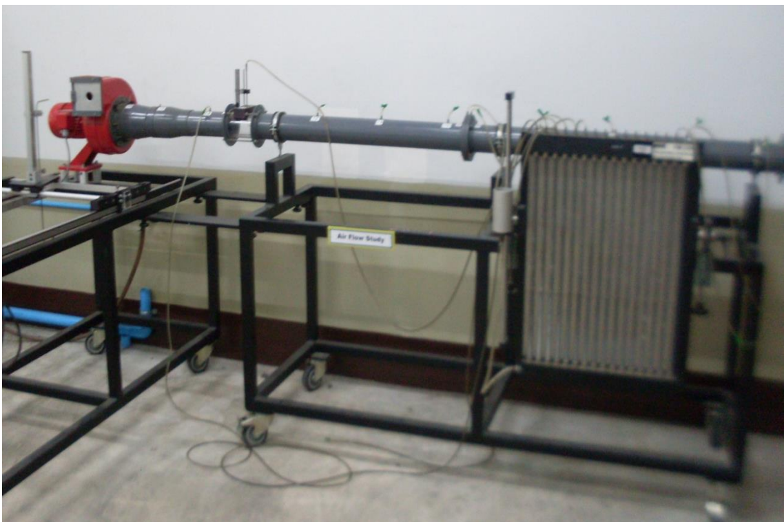
Air Flow Test Set
