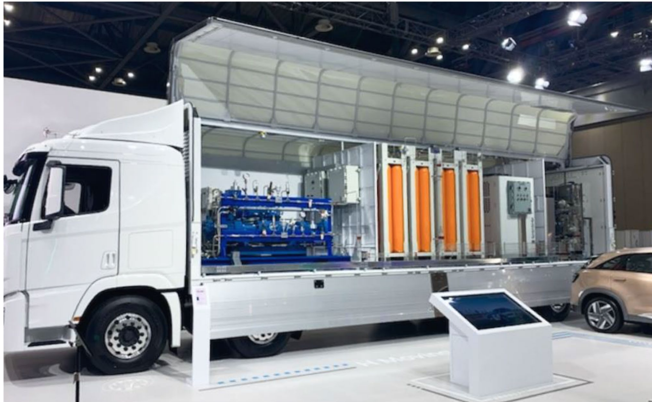
Hydrogen Production Modules (SMR : Steam Methan Reformer)
